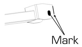
Mark the rear frame rails along the edge of the connector. This will show you where to grind the paint/grime off the frame. Don't forget the outboard tab. This area will be difficult to access since the leaf spring and bracket are in the way.
