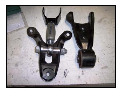
9. Install first the two (2) bolts from the upper mounts by having it finger tight, and then install the third bolt for the upper mount under the rear seat.
