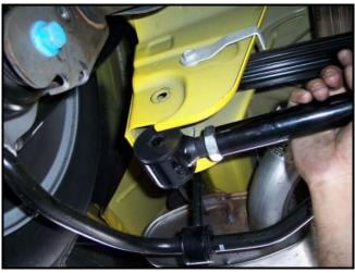
Reuse the stock hardware to fasten the driver side mount. Do not fully tighten at this time.
