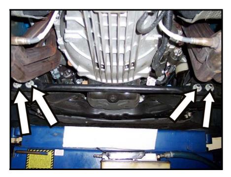
2. Install the new under brace by hand tightening the four (4) nuts/bolts. If only holes are there use supplied 12mm X 30mm bolts, nylock nuts, and washers.
