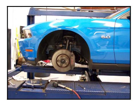
2. Remove the brake line bracket.
