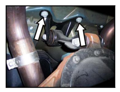
7. Remove the lower mounting bolt of the upper trailing arm to the differential.
