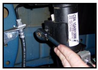
5. Loosen the nut on top of the strut underneath the hood.
