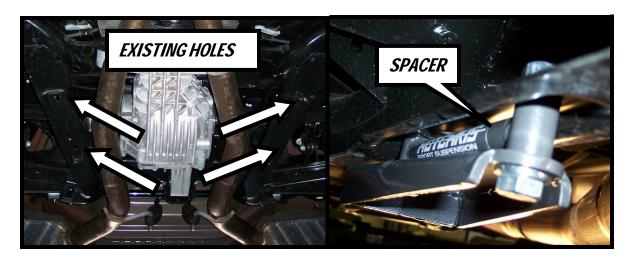
4. The Front bracket should now line up with its hole. Use the provided hex bolt and LARGE washer on that bracket.
