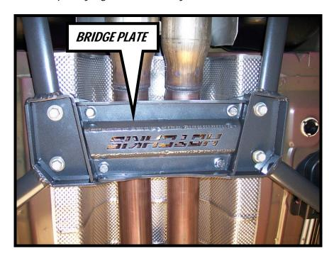
7. Once everything has been bolted on, begin tightening the bolts on the outside main braces. Tighten M10 bolts to 50 ft-lbs and M12 bolts to 90 ft-lbs.
