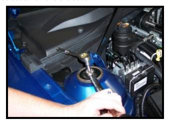
6. <u>Mark the strut where the upright nuts are located with a marker</u>. Remove the bolts that hold the spindle to the strut.
