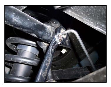
3. Disconnect the OE end link from the front struts. Retain the nut for reinstallation.
