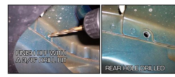
10. Once the rear holes are drilled out on the both sides, Position the strut brace in the engine bay. Install the longer rear bolts through the holes you just drilled and through the rear bracket of the brace. Spin the nuts on, but do not tighten. The front mounts will sit in front of the strut towers.
