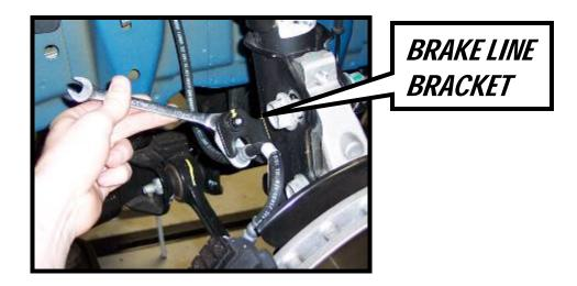
3. Remove the ABS line from the bracket.
