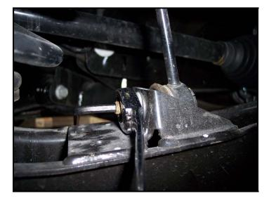
4. As a default setting, set the length of the Hotchkis links to the same length as the OE links. Tighten the jam nuts once the length is set.
