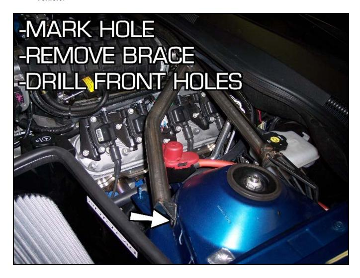
12. Drill the front holes in the same manner as the rear holes. Start with a 1/16" or 1/8" pilot hole and finish it off with a 3/8" hole. These holes can be drilled from the engine bay side.
