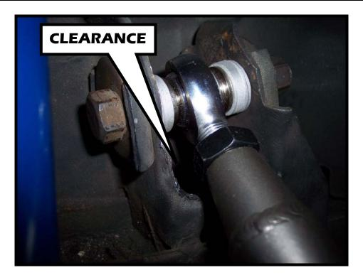
9. Install the new A-Arms by following the same instructions in reverse order. When bolting on the rod ends, be sure to use the provided spacers.
