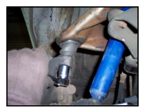
3. With the castle nut loose, hit the upright mount with a hammer until the spindle & the rest of the suspension pop loose from the A-Arm ball joint.
