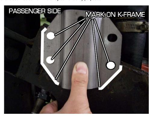
Once the k-frame is marked, use an angle grinder with a sand paper attachment to remove all of the paint and grime on the areas previously marked. What we are doing is cleaning the area that is going to be welded.
