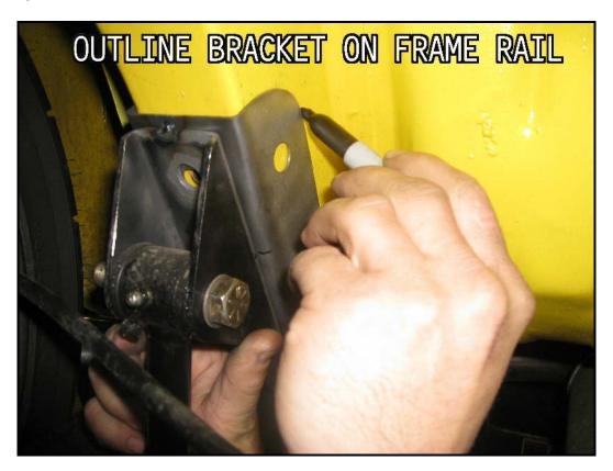
With the brackets in position, mark the hole position of the triangle bracket onto the reinforcement bracket.
