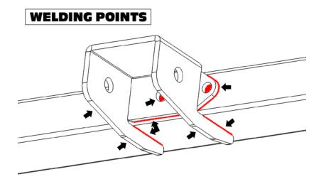
When you're done welding the front mounting bracket, reinstall the subframe connector. Fully tighten the 4 rear mount nuts. You may now remove the jacks supporting the rear subframe. The full weight of the car should be on all four tires from now on. Use the screw jack once again to hold the subframe in place if need be. Now weld the subframe connector to the front mounting bracket.
