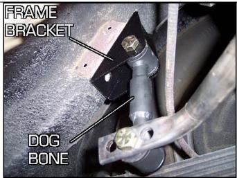
We've noticed on some E-bodies that the distance between the left and right frame rails were ½" wider. If the frame bracket does not line up in the center of each frame rail due to the frames having a wider span, then please install the optional spacer between the sway bar and the end link.
