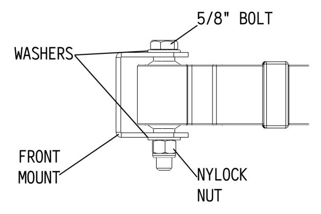
Diagram shows Driver Side with the 5/8" bolt pointing outboard.
