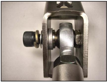
Stack Up: 3/8" bolt---Split Lock washer---AN Washer---Relocator--0.185" Spacer---Misalignment Spacer---Heim Joint
