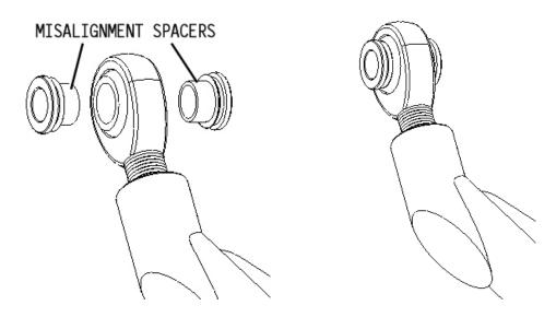
Position the A-Arm so that the other heim joint is lined up with the mounting hole. You will notice there will be gaps on each side of the joint. You will need to add spacers (included in your kit) to take up the gaps. These gaps are not consistent from car to car so you will have to use the appropriate thickness spacers on each gap. You may have to use combinations of varying thicknesses to achieve proper gaping. See below as an example.
