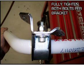
Now you can raise the bar up until the bushing retainer brackets mate flush to the k-frame bottom surface. Make sure the center section of the sway bar is not contacting any part of the k-frame. Bushing retainer bracket should be positioned similar to the picture below. The white outline depicts the k-frame. (Picture shows bracket disconnected from the sway bar for clarity
