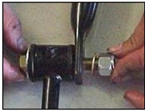
Use the grease pack to also apply a thick coat of grease to the insides of the sway bar bushings. Place the bushings over the bar with the split of the bushing facing towards the rear. Install the bushing retainer brackets over the bushings.
