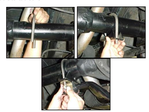
8) Use the tube of anti-seize included with the kit to apply a small amount to each set of threads on the u-bolt. **DO NOT** tighten the nylock nuts without using anti-seize! You could ruin the nuts or snap the u-bolt without it.
