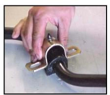
Attach the triangle brackets to the stud plates on the frame. Tighten the attaching hardware, as this is easier to do before installing the sway bar. With the brackets attached to the frame the bar can be lifted into place. Connect the end links to the brackets. The sway bar should be hanging loosely from the brackets at this point.
