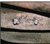
Use the grease pack provided with the kit to apply a thick coat of grease to the sides of the dog bone end link bushings. Attach the end links to the sway bar on the outside of the sway bar ends. Install the hardware with the bolt head towards the outside of the frame. The larger washer should be against the bushing and the smaller washer will be to the inside against the sway bar. See the picture below for assembly.
