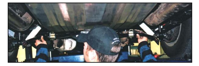
Place the u-bolts over the rear axle. Slide the axle brackets over the ends of the u-bolts with the curved side up against the axle. Rotate the bar into position and slide the bushing retainer brackets over the ends of the u-bolts. Start the nylock nuts onto the ends of the u-bolts to loosely hold the bar to the axle.
