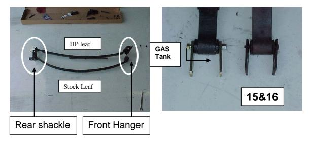
16. Install the leaf springs. You need to set the vehicle on its wheels before you perform the final tightening on the leaf spring eyelet bolts. You must do this so you don't ruin the leaf spring bushings.
