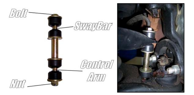
9F. Using the included white silicon grease, lube the inside of the new 1 <sup>1</sup>/<sub>4</sub>" front bushings. *NOTE: the grease can be cleaned up with WD-40*
