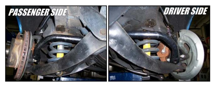
8F. Once the bar is in place, install the new endlinks but do not tighten them completely.
