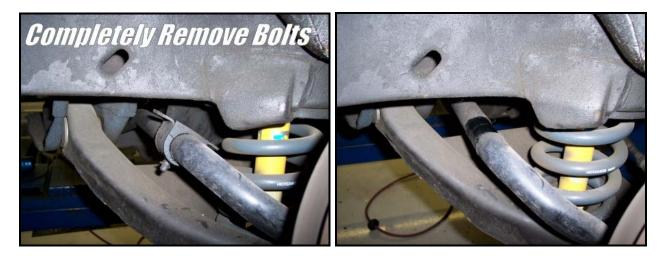
6F. Turn the steering all the way to the LEFT and remove the stock bar through the DRIVER side wheel well. Observe the following pictures for the removal procedure.
