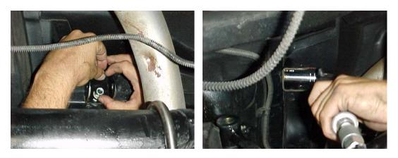
14) Re-attach the end links to the brackets, and tighten all attaching hardware on the end links.
