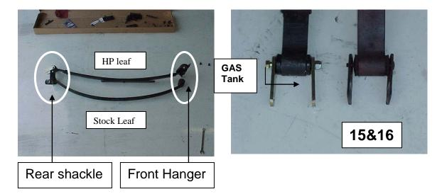
17. Install the leaf springs. You need to set the vehicle on its wheels before you perform the final tightening on the leaf spring eyelet bolts. You must do this so you don't ruin the leaf spring bushings.
