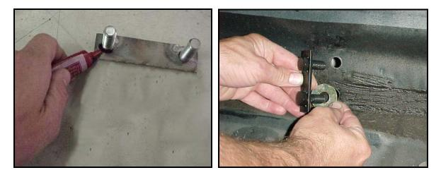
13) Remove the triangle brackets from the end links. Attach the brackets to the stud plate with the large end of the bracket closest to the ground. Tighten the hardware holding the bracket in place.
