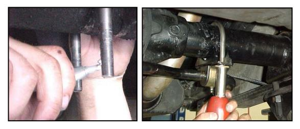
11) Rotate the sway bar into place with the triangle brackets up against the body. Use a scribe or other marking tool to mark the locations of the holes on the body matching the bracket. Drill out two 1/2" diameter holes on each side to match the bracket locations.
