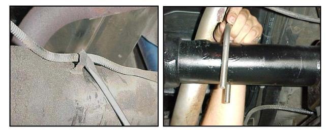
9) Lift the bar assembly into place under the rear of the car with the arms of the bar pointing forward. Use the axle mount brackets provided to hang the sway bar loosely from the axle. Slide the u-bolts as necessary to center the sway bar on the axle.
