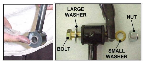
7) Use the shorter length bolts (2-3/4") from **hardware kit #T1712** to attach the triangular bracket to the end links. *The larger end of the bracket should be closer to the ground when installed.* Loosely start the hardware so that the assembly can rotate freely.
