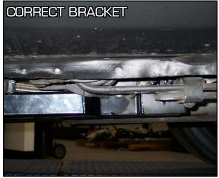
The other bracket we have encountered drops the front eye below the visual line of the rocker seam. This will cause an unwanted increase in ride height and our springs were not developed for use with this type of bracket. Please purchase the standard leaf spring mount from your local parts supplier to correct this issue.
