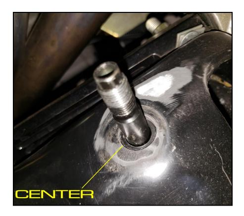
Install the rubber bushing, washer plate, and lock nut onto the shaft thread. Tighten lock nut until the rubber bushing begins to bulge. Do not over tighten.
