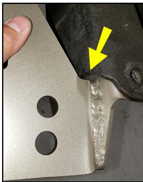
Mark the center of the slot to drill a 3/8" hole. You can remove the bracket if it gets in the way of drilling.
