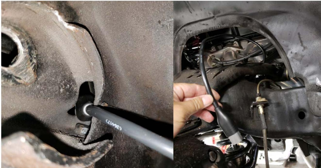
\*SPECIAL NOTE\* Make sure the Delrin bushing's centering boss is perfectly centered in the 3/4" upper hole. It is very easy to misalign the bushing when fastening the top nut
