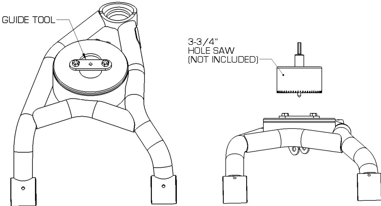
Use the upper retainer plate as a template for the remaining cut out shape. Mark the arm to cut out the square sections. Note the clocking orientation of the cut out shape.
