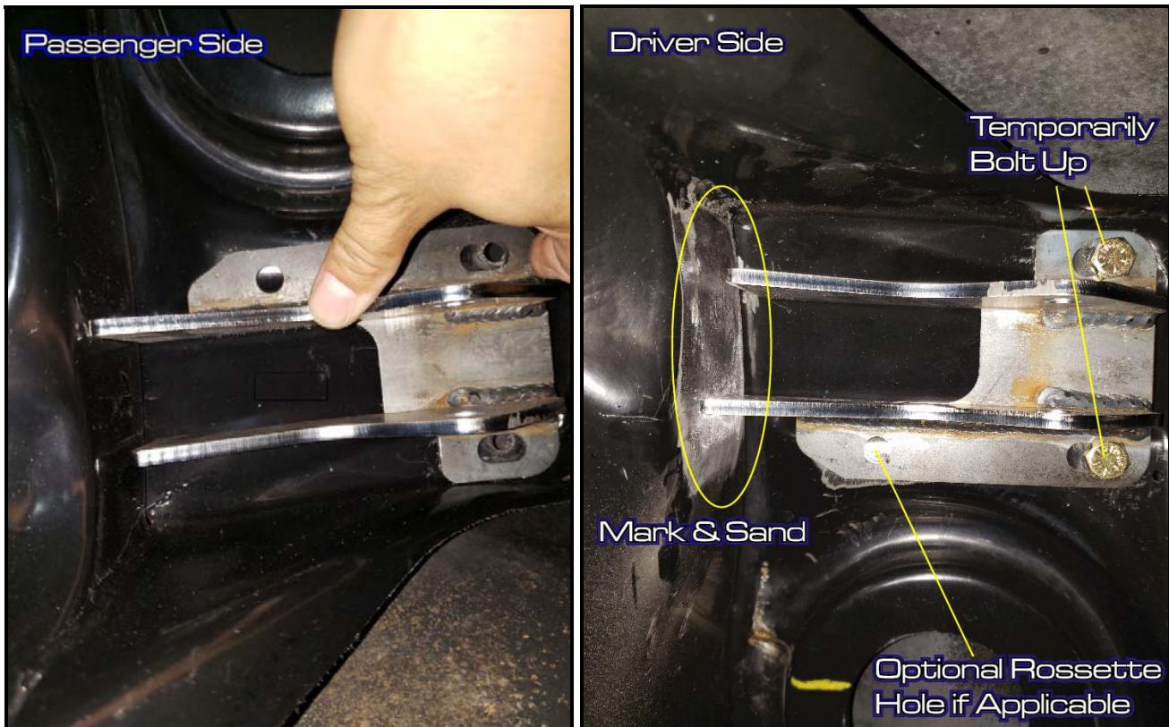
Also sand the gusset wall edges on the Hotchkis brackets. About 3/4" in from the edge should be enough sanding area for the weld. There is an optional rosette hole in the bracket if your frame mates flush with it. If desired, you can sand the powder coat off the hole area for welding as well.
