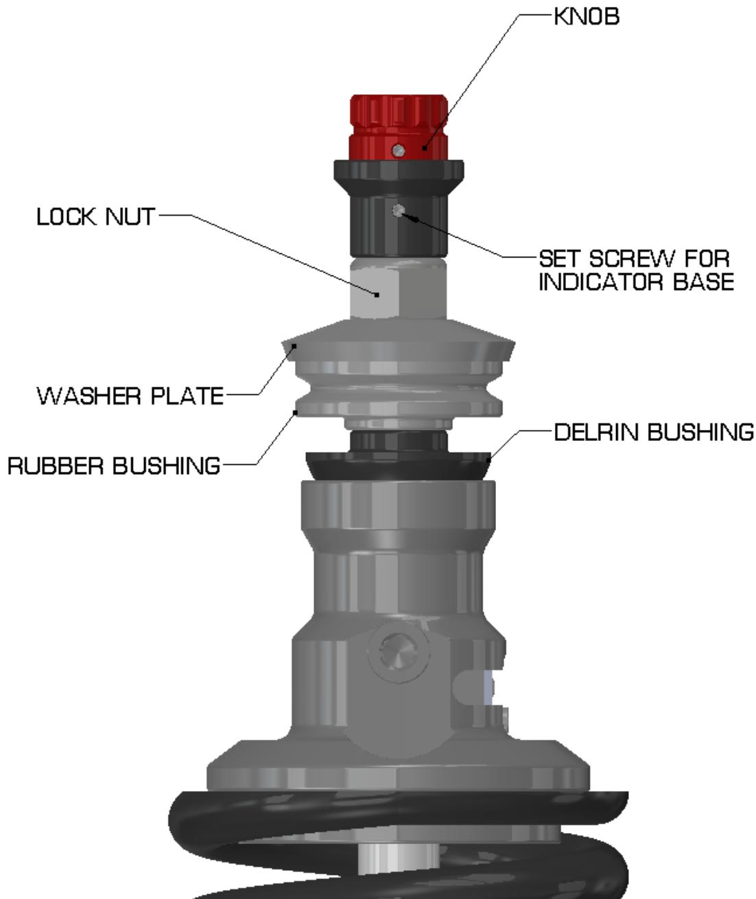
Insert the coilover thru the access hole in the lower a-arm. Guide the upper mount up to the 3/4" shock hole. You may need to adjust the suspension assembly up/down travel to allow this.
