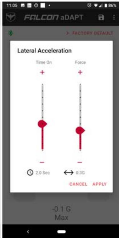
**G-Force Threshold:** This is the setting that dictates when the "Performance" mode is activated.
