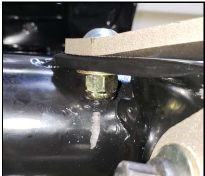
The bracket also utilizes the original shock mount hole. In some cases you will need to use spacer(s) in between the axle bracket and the hotchkis bracket. Use the provided spacers to take up the gap. Use the 1/2"-20 x 1.75" bolt to secure this mounting point.
