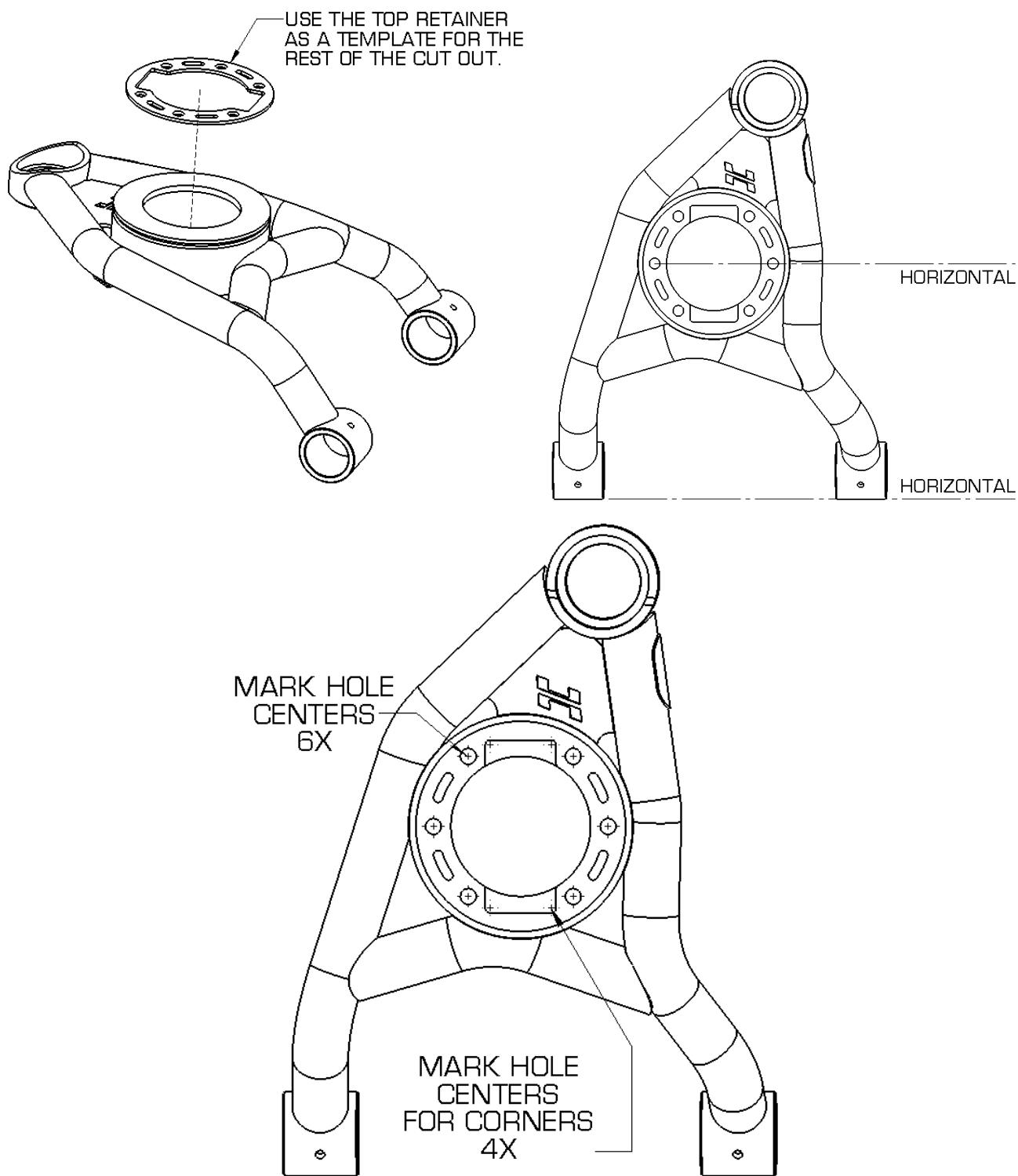
Use a 1/4" drill bit on the corners of the square cut outs.
