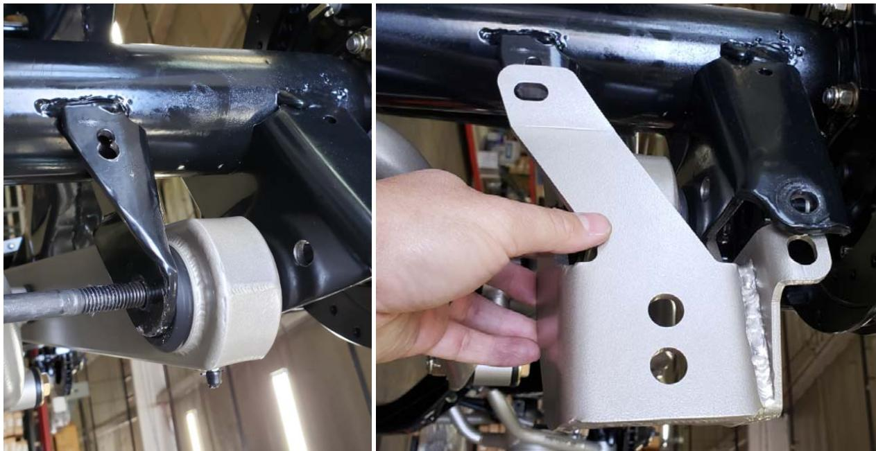
In some cases, you may need to clearance the bracket on the axle to allow the lower mount to fully rotate up.
