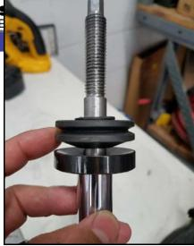
Guide the shaft to line up with the top shock hole.
