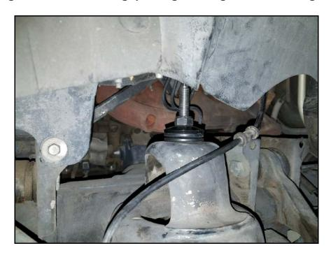
Reinstall the ABS clamp, ABS line, and wheel. Lower the truck and you are done with the front.
