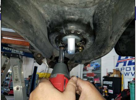
From the top, Install the remaining bushing, retainer and lock nut onto the shock shaft. Tighten until the bushings just begin to bulge. Do not over tighten.
