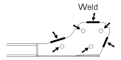
If you find that the rear section of the bracket has too much gap between the bracket and the frame rail, you can use vise grips to squeeze the sides together to take up the gap. Likewise, if you have too much gap between the bottom of the bracket and the bottom of the frame rail, then you can use a hammer to slightly bend the bottom portion of the bracket up to close the gap. The bracket was designed with reliefs at the bend area for this purpose.
