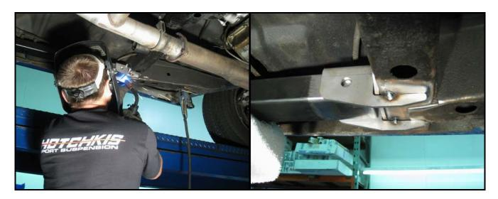
Once the position is confirmed weld the entire bracket to the frame.
