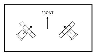
Step 1: Place the tool on the front of the bushing mount and the large disk on the rear.
