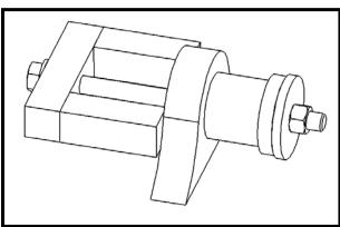
Step 2: Tighten the nut until the bushing is pressed securely into the mount. The bushing will not be pressed all the way to the flange due to the increase in diameter of the can. This is normal.
