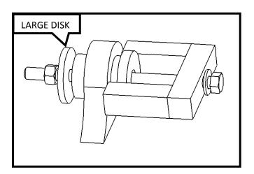
Step 2: Tighten nut until the large disk is up against the bushing mount.
