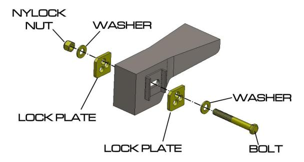
The Hotchkis plates have a unique shape with a chamfer on one corner and a large radius on another. The last (2) corners are sharper corners. This shape allows for easy identifying to insure the clocking is the same for each pair of plates. Just remember chamfer goes with chamfer and radius goes with radius. Your holes will always line up.
