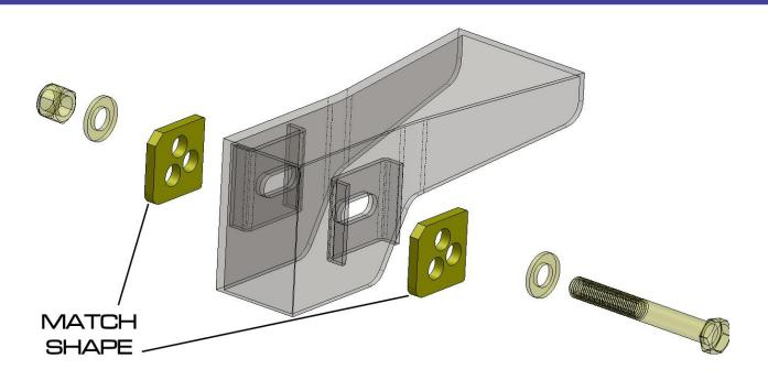
Once the 1/2" bolt is fully tightened, you are finished and can rest assured knowing your alignment is locked down will not creep.
