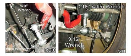
(Step 3) Next, center the ball joints to avoid possible binding. Once they are positioned, tighten the jam nut using an 11/16" wrench. Use vise grips to hold the female ball joint to avoid spinning.
