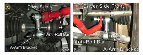
(Step 2) Use a 9/16" wrench and a 3/16" allen wrench to tighten the nylock nuts for each stud. (*Tip: If possible, try using a "ratcheting wrench" to speed up the process.*)
