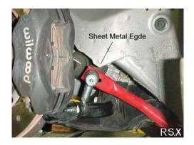
Use a hammer to bend the edge inboard as shown in the following picture.
