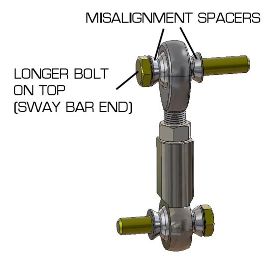
6. Reinstall the Hotchkis end links onto the vehicle in the same manner as removal. Reuse the OE nuts. Tip: Use blue thread locking compound on these nuts. Tighten the jam nuts once the length is set.
