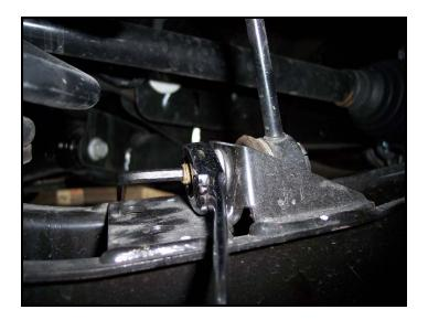
4. As a default setting, set the length of the Hotchkis links to the same length as the OE links. Tip: Use blue thread locking compound on these nuts. Tighten the jam nuts once the length is set.
