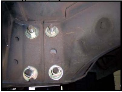
7. Now remove the lower nut on the rear bracket and slide the leaf spring off the bracket bolt.
