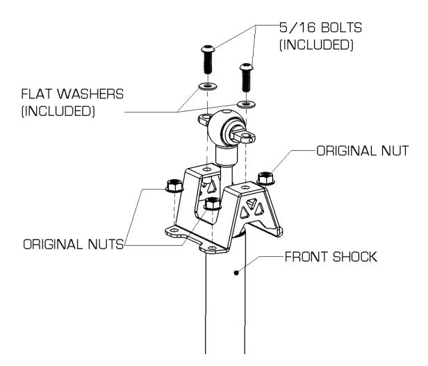
Special Note: If you have our existing Hotchkis APS shocks which came with height spacers for the shock t-bar, please discard them for this install. The new bracket design is slightly taller and has a larger window for the adjuster knob which eliminates the need for these spacers.
