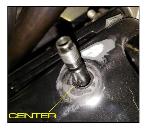
Install the rubber bushing, washer plate, and lock nut onto the shaft thread. Tighten lock nut until the rubber bushing begins to bulge. Do not over tighten.
