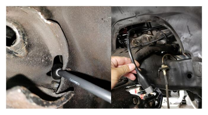
\*SPECIAL NOTE\* Make sure the Delrin bushing's centering boss is perfectly centered in the 3/4" upper hole. It is very easy to misalign the bushing when fastening the top nut
