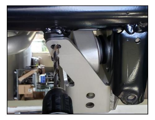
Reinstall the bracket with the 1/2"-20 x 4.25" hex bolt, washers, and nylock nut. Install the 3/8"-24 x 1.25" button head bolt with no washer on the head side. Use the 5/16 USS washer and 3/8"-24 nylock nut. Keep the nuts loose for now.
