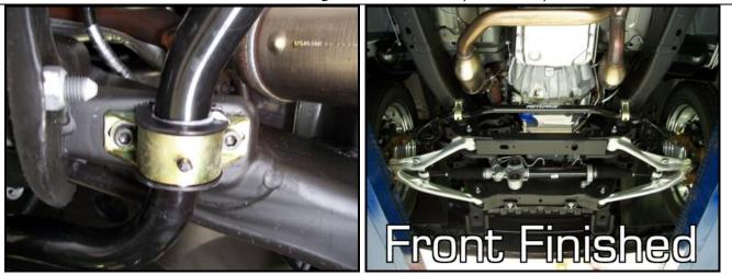
The flat cut washers should fit tight onto the socket bolts. You may need to wiggle the washers onto the bolt to install.
