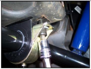
The flat cut washers should fit tight onto the socket bolts. You may need to wiggle the washers onto the bolt to install.
