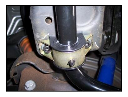
Reattached the stock end links to the Hotchkis sway bar ends.
