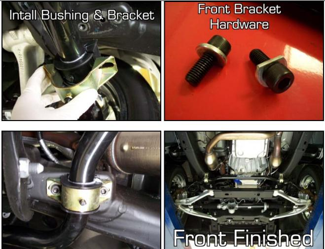
The flat cut washers should fit tight onto the socket bolts. You may need to wiggle the washers onto the bolt to install.
