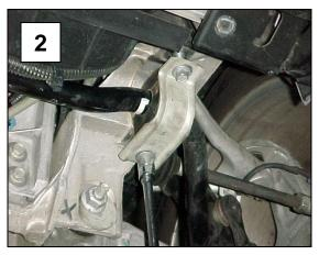
Once you disconnect everything pop the lower end link stud out of the holes, slide the bar sideways and twist it out of the vehicle.
