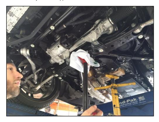
12F Unbolt the (6) mounting bolts securing the subframe to the chassis. Lower the subframe to access the front sway bar.
