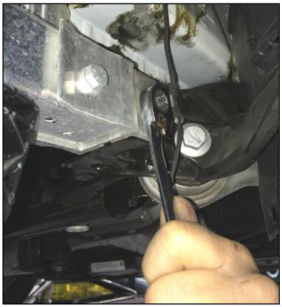
7F Remove the (3) bolts per motor mount.
