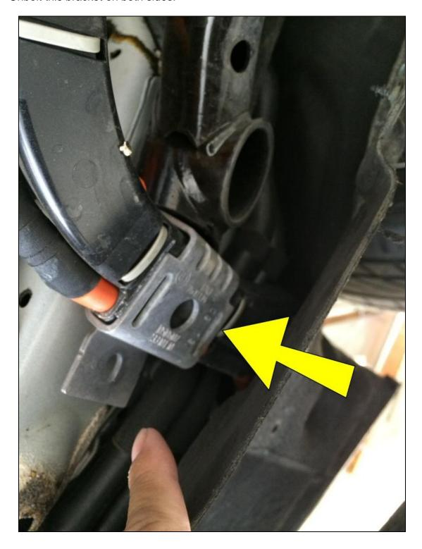
13F Unbolt the bushing bracket nuts. (2) nuts per bracket. Retain these nuts for later use.
