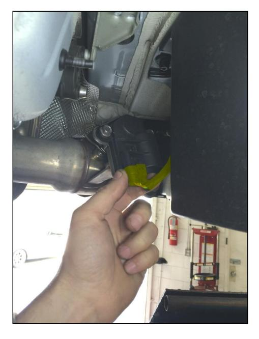
6R Unclip the wires attached to the upper link.
