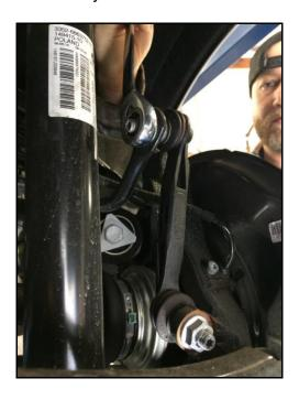
8R Remove the lower shock mount bolt.
