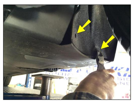
Next, remove the push-in rivets that secure plastic panel itself. This exposes the front support brackets for the subframe.
