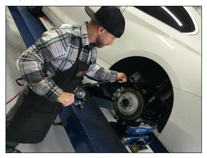
15R Place the OE bar next to the Hotchkis Bar to orientate the new bar.
