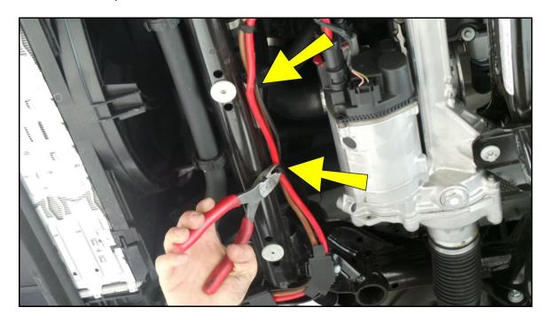
Next, disconnect the small connector and large connector from the power steering unit.
