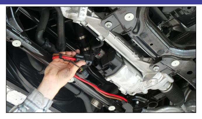
Pull the plastic wire carrier out of the way.
