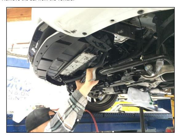
14F Place the Hotchkis bar next to the OE bar to compare. Grab the Hotchkis front bushings (larger pair) and grease the inner surface with the provided lube.
