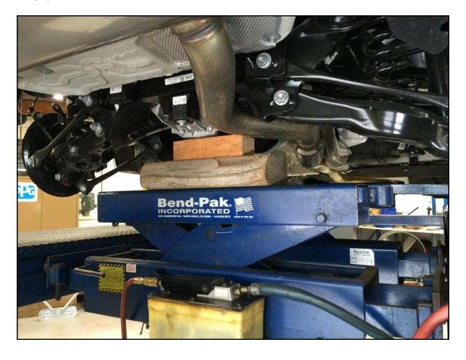
11R Unbolt the subframe from the vehicle. There are (2) support brackets holding up the front and (2) subframe bolts securing the back.
