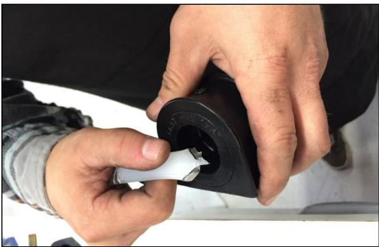
15F Install the bushings onto the bar as shown below.
