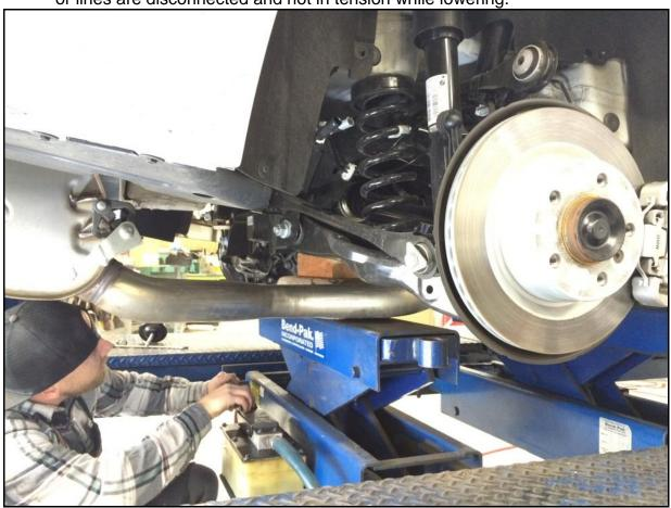
13R With the subframe lowered you are now able to undo the (2) bolts per bushing bracket on each side. Retain these bolts for reinstallation.
