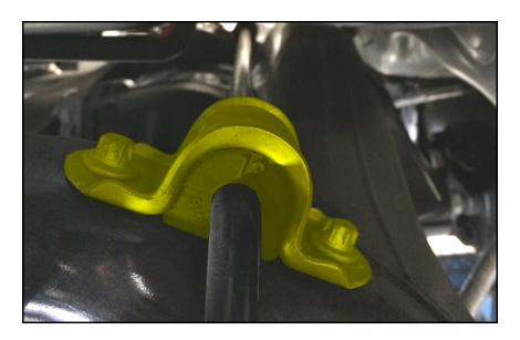
14R Fish the rear sway bar out from the vehicle. Take note of the orientation of the bar as you remove it.
