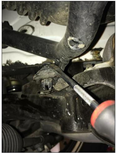
Remove the plastic center side panels. Both sides.
