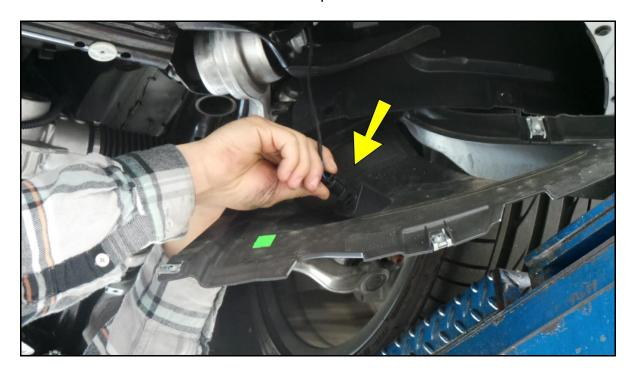
Pop the plastic push-in rivet holder from the subframe. (Note picture shows subframe already dropped for clarity.)
