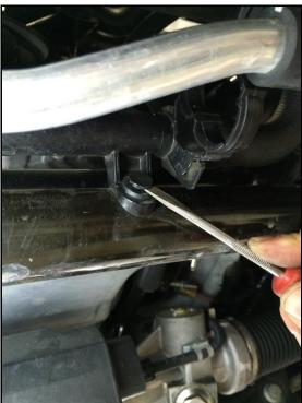
6F Remove the (1) bolt attaching the subframe rail to the aluminum radiator support. (1) bolt per side.
