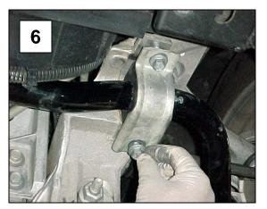
7. Tighten the frame mounts using a 15mm socket, wrench and extension. Torque to 35-40 ft-lbs.
