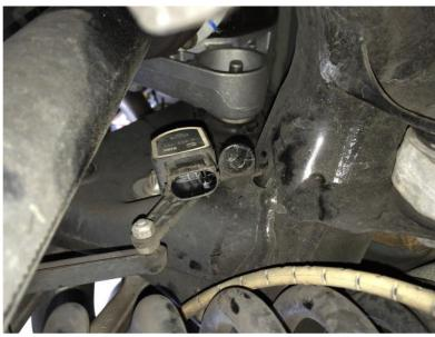
10R Disconnect the Hold Down Bracket on Upper Link
