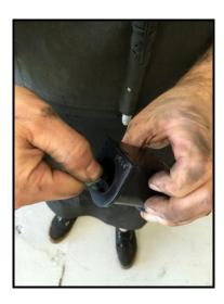
Open up the bushings at the split and install onto the bar near the intended bushing location. Install the Hotchkis bushing bracket onto the bushings and mount to the chassis. Make sure the 90° grease fitting on the Hotchkis bracket is facing outward. If the fitting is not facing the correct angle, it can be tighten to adjust to face in the right direction. Use the included Hotchkis washers with the OEM nuts to secure the bracket to the chassis.
