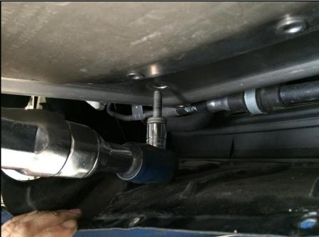
Remove the aluminum splash pan and set aside.
