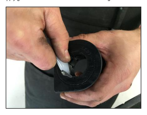
Open up the bushings at the split and install onto the bar near the intended bushing location. Install the Hotchkis bushing bracket onto the bushings and mount to the chassis. Use the included Hotchkis washers with the OEM nuts to secure the bracket to the chassis.
