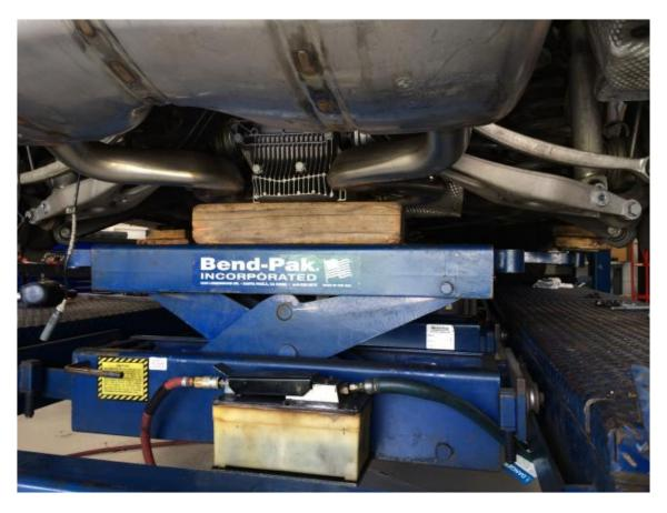
Unbolt the forward mounting bracket on each side. This will take care of (2) of the (4) main subframe bolts holding up the subframe.
