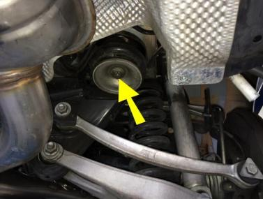
The subframe can be lowered down. Lower the subframe slowly watching for any wires that might be snagging or pulling. If you see any wires in tension, then raise back up and disconnect the wires to free up some slack. You only need to drop the subframe enough to snake the rear sway bar out from either side.
