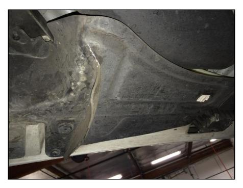
Once you have these plastic panels removed you should have a clear shot at the forward mounting bracket for the rear subframe. We will get to this later in the procedure.
