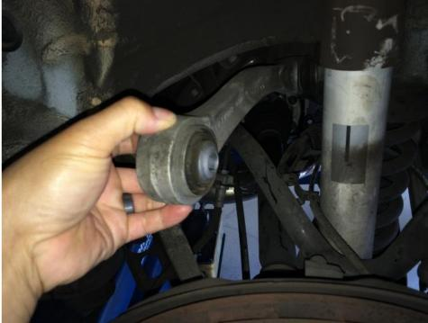
12R Disconnect the Lower Shock Mount Unbolt the lower shock mount.
