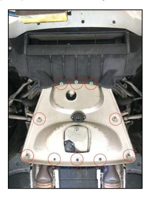
Start by undoing the fasteners that secure the front felt cover to the pan. You want to be able to pull down on the felt cover to access the bolt holding the front of the aluminum splash pan.
