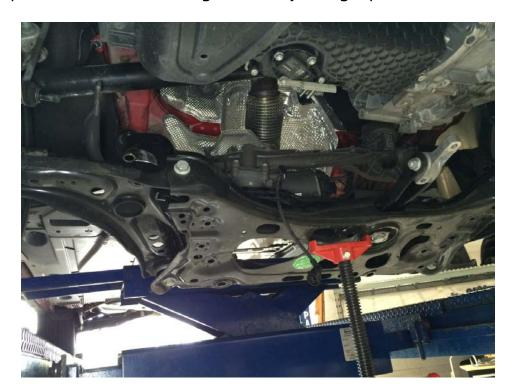
You will notice a plastic holder that is clipped into the subframe. Use a screw driver to pop the plastic push-in rivet out to release the plastic holder.
