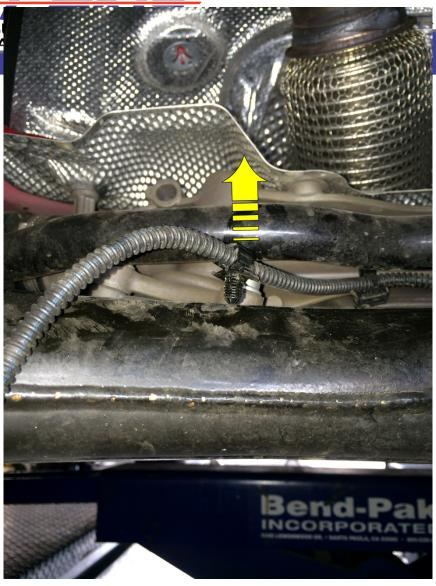
The subframe should be able to drop down quite a bit to allow the sway bar to be removed. If it doesn't, the steering rack assembly might be stuck onto the subframe. Gently pry and wiggle the assembly away from the subframe. Sometimes raising the subframe back up can help dislodge the steering rack from the frame.
