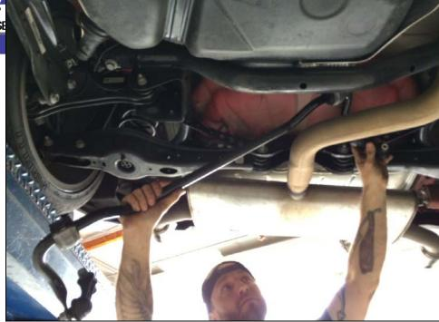
5R Place the OE bar next to the Hotchkis bar and transfer the end links over. Use the 6mm Triple square socket to hold the end link stud.
