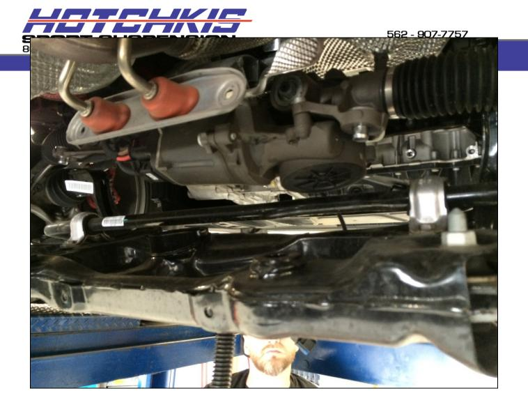
12F Remove the (2) bolts for each bushing bracket and remove the bar from the car. Note the orientation of the stock bar as it comes out.
