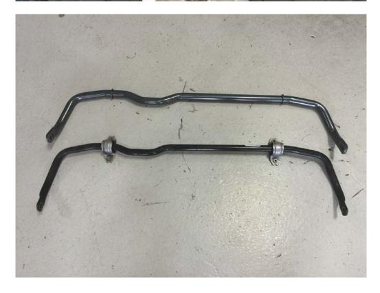
13F Grease the Hotchkis polyurethane bushings with the provided lube. Install bushings on the bar as shown below.
