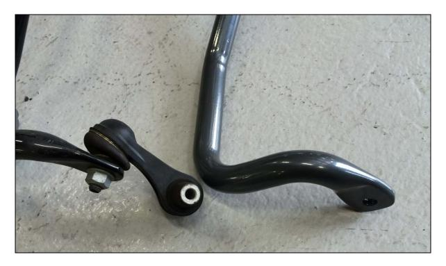
Use blue loctite on the end link studs.
