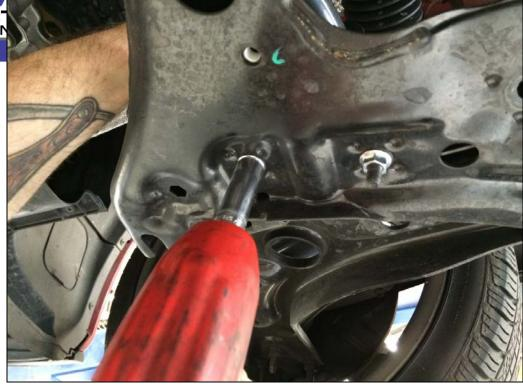
15F Begin raising the screw jack to bring the subframe up back to the subframe. You will need to guide the steering rack assembly back to its home on the subframe as you go up.
