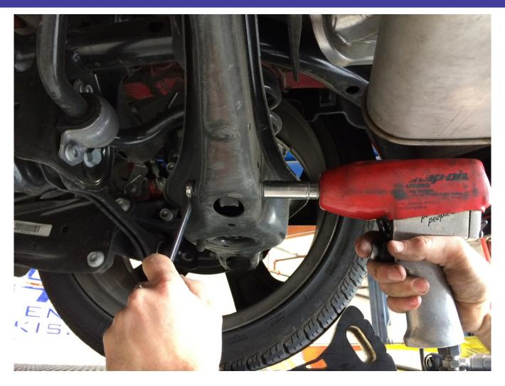
3R Unfasten the (2) bolts from each of the bushing brackets using a 10mm triple square socket tool.
