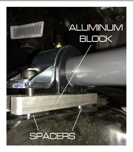
Fully tighten the bushing bracket hardware at this time.
