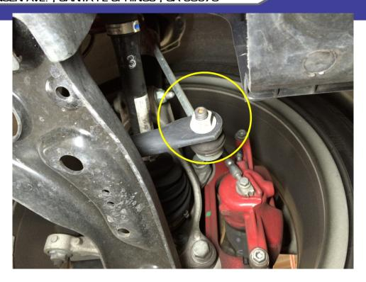
3F Disconnect the lower dogbone mount at the engine. Unfasten the (2) bolts to the engine and loosen the large bolt at the subframe mount
