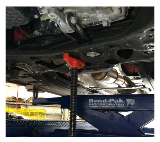
Remove the (4) bolts that hold the subframe to the chassis.
