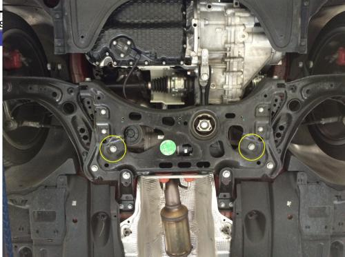
7F Remove the (2) smaller bolts on each rearward subframe mount.
