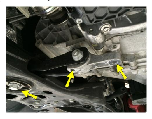
4F Unfasten the (2) bolts securing the exhaust mount to the subframe.
