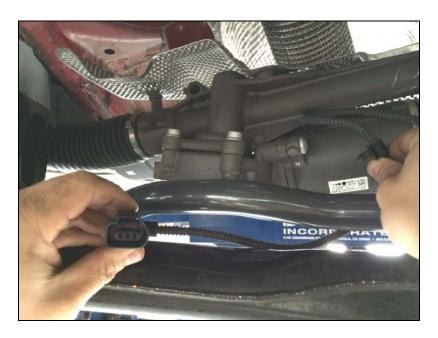
Tip 1: Be patient when lining up the steering rack with the subframe. The steering rack has dowels that positions itself to the subframe. Do not force the mounting bolts to screw in. They should screw in by hand most of the way. To be safe, you can use anti-seize to avoid galling the threads during this process.
