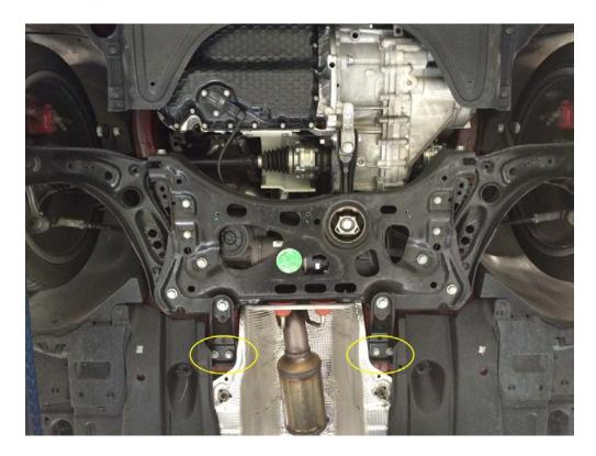
8F Raise the front of the vehicle at the jack points until the wheels begin to lift off the ground.
