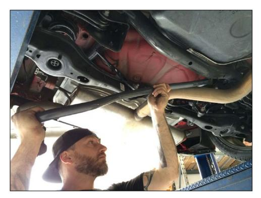
7R Reinstall the end links back onto the lower control arms. Fully tighten this hardware.
