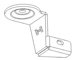
Undo the rearward subframe bolt (one at a time). You may discard the large washer. Install the correct side bracket onto the bolt and fasten it back into place.
