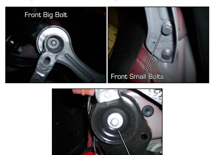
Carefully lower the sub-frame down with the jack until you can access the sway bar bushing brackets. Be careful not to lower the sub-frame too much, or damage to the brake lines will occur.
