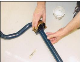
6/ Lift the bar up to the vehicle with the two smaller H-Sport stickers at the ends right-side-up. As you lift the bar up to the mounting points, <u>you must place one mounting plate per side between the bushing and the mounting point.</u>
