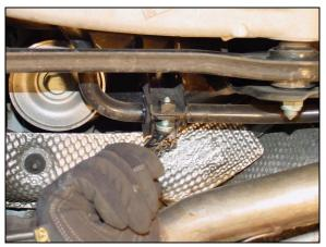
6/ As you begin to remove the bar, gently free each end from the end link sleeves. Now that the bar is free, slightly lower the exhaust by applying pressure to the tips just enough to remove the bar towards the front or the rear of the car.
