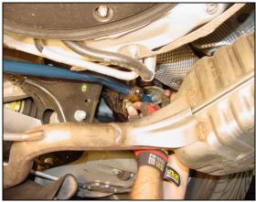
9/ Re-install the four stock bracket bolts, **include the four supplied washers**, to the new brackets and leave loose while you insert the small end link sleeve to each end of the bar. Re-install the end link bolts and leave loose. Tighten the four bracket bolts, then tighten the end links bolts. Six bolts, all tight.
