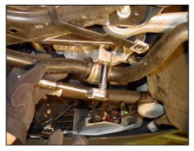
5/ Apply second tube of grease to each inner-channeled portion of the two new front bushings and attach to Hotchkis bar against the outside of the washers. Slip the new brackets over the bushings.
