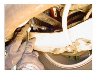
5/ Remove the four bushing bracket bolts (13mm wrench) attaching the antiroll bar brackets to the sub-frame and save them.
