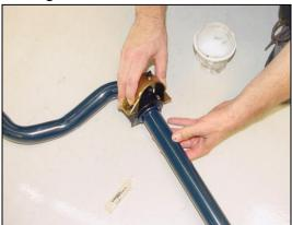
6/ Lift the bar up to the vehicle with the two smaller H-Sport stickers at the ends right-side-up. As you lift the bar up to the mounting points, <u>you must</u> <u>place one mounting plate per side between the bushing and the mounting point.</u> This relocates the bushing out of the stock bushing pocket. Re-install the bracket nuts and tighten. <u>Re-install the end link bolts and tighten well using medium strength thread locker</u>.
