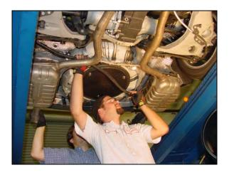
7/ Repeat same pressure to the exhaust and position Hotchkis bar (without the bushings and brackets) in the stock location with the Hotchkis sticker facing
