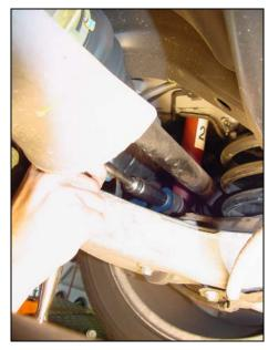
\*Adjustability Note: choose the inner hole (2<sup>nd</sup> from bar end) for a more aggressive feel and the outer for solid front-to-rear balance. Loosen the lower end link bolts(2 under cast arm each side) on the bottom side of the lower arm in order to adjust to desired hole.
