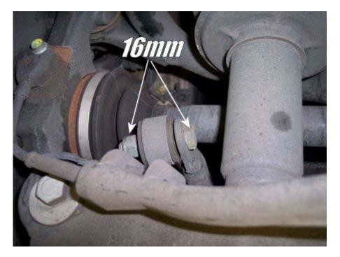
7) As you begin to remove the bar, gently free each end from the end link. Now that the bar is free, you can snake the sway bar through the exhaust pipes.
