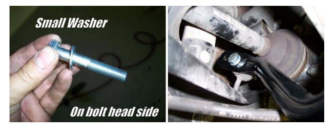
Adjustability Note: To adjust between the two holes, you must unbolt the bushing bracket bolts and pull the bar towards the rear so that the end link bolts clear the shock bodies. The hole at the bar's end is the normal setting, while the second hole from the end is the stiffer setting.
