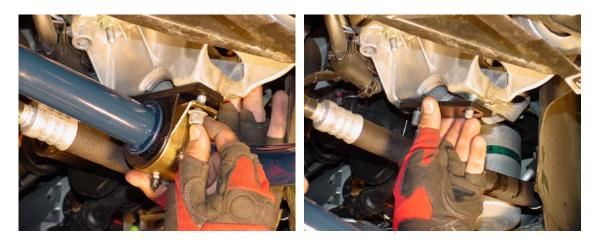
7/ Re-install the bracket nuts and tighten. <u>Use a small portion of blue thread-locker on the</u> <u>end-link bolts</u>, re-install and tighten well. \*\*Note\*\* If vehicle is raised using jack stands or other, the bar end and the end link may not align properly. Lower vehicle so that front suspension is not at full droop and ends will align. <u>Be sure to thread end link bolt by hand at first to prevent</u> <u>cross threading</u>.
