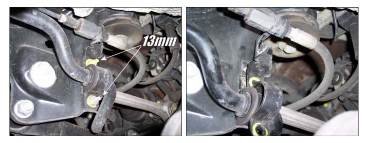
6) Remove the two end link bolts and nuts (16mm wrench) which attach the bar ends to the end links and save them. To clear the shocks with the bolts, pull the bar towards the rear of the car.
