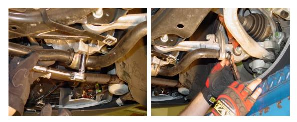
5/ Apply a quarter tube of grease to each inner-channeled portion of the two new front bushings and attach to Hotchkis bar against the outside of the washers on the bar. Slip the new brackets over the bushings.
