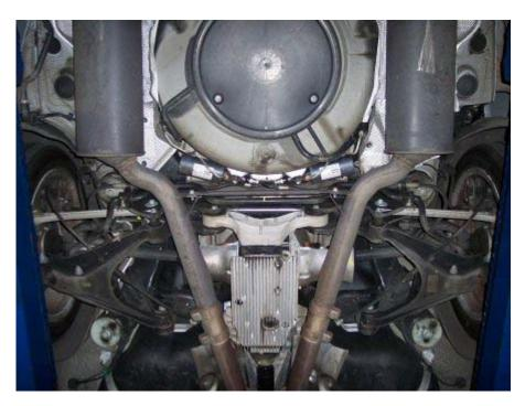
3) Undue the rear exhaust hanger brackets and middle hangers then let hang. Use WD-40 to loosen the rubber hangers. Unbolt the hanger brackets using an extension and 13mm socket. It's a good idea to support the exhaust system (e.g. near the tips) once you've achieved the desired space needed to remove the sway bar. This will avoid bending the exhaust system down more then needed.
