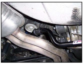
Next, slide the bushing brackets over the bushings. Position the bracket onto the stock mounting point. You will need to install the provided aluminum reinforcement plate on the backside of the mount. Fasten the bushing bracket and reinforcement plate together using the provided hardware.
