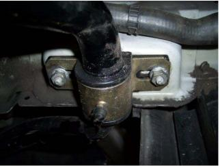
5) Apply grease along the inside surface of your polyurethane bushings and attach them to the Hotchkis bar in the approximate mounting locations. Slip the new brackets over the bushings.
