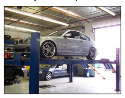
2) Once the vehicle is raised, use a Phillips screwdriver and remove the aero-pan fasteners. Let the pan hang from the front in order to expose the stock front sway bar.
