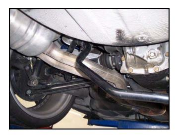
Pay close attention to the way the stock end links are mounted to the brackets. These brackets will be used to mount the new end links to the upper cast arms. Remove the stock end links from these brackets and then mount them to the H-Sport end links using the stock hardware. Pay close attention to zerk fitting direction. The lower Zerk Fitting points towards the rear of the car.
