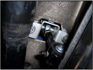
9) Apply grease along the inside surface of your polyurethane bushings. Install the rear bushings onto the bar at the approximate mounting location. Now you may install the Hotchkis rear bar with the H-Sport sticker facing the rear, right side up.
