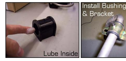
Apply a small amount of anti-seize to the threads of the U-bolts. Next position the axle bracket up against the axle tube. Raise the sway bar up to meet the axle bracket and allow the U-bolts to poke through the bushing bracket. Fasten the assembly together with the provided nut and washer. Do not fully tighten.
