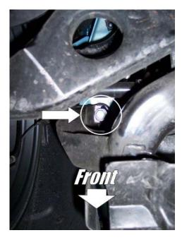
d) Finally, using the same 16mm socket, remove the 4 bolts (2 per side) at the front of the sub-frame where it slips into the two solid frame points.
