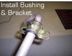
Apply a small amount of anti-seize to the threads of the U-bolts. Next position the axle bracket up against the axle tube. Raise the sway bar up to meet the axle bracket and allow the U-bolts to poke through the bushing bracket. Fasten the assembly together with the provided nut and washer. Do not fully tighten.
