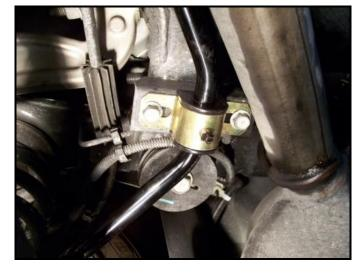
» Reattach the end links to the sway bar ends using the stock hardware. Fully tighten end link nuts. Note: 2280A Kits have (2) hole adjustability. The hole closest to the end is the soft setting.
