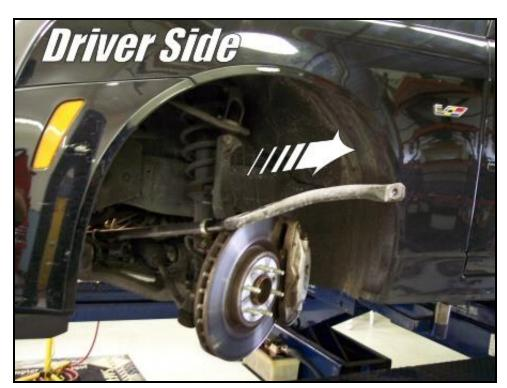
» Place the stock sway bar on the floor and set your new Hotchkis sway bar next to it. This will allow you to properly orient and position the bar for reinstallation.
