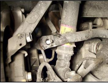
Peek inside the wheel well and locate the subframe mounts. You will have to undue 2 bolts per side.
