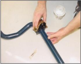
6/ Lift the bar up to the vehicle. The two smaller HSport stickers at the bar's ends should be right-side-up. As you lift the bar up to the mounting points, <u>you must place one mounting plate per side between the bushing and the mounting point.</u> This relocates the bushing out of the stock bushing pocket.
