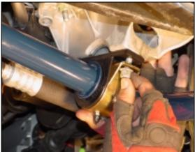
7/ Re-install the bracket nuts and tighten. Apply Blue threadlocker to the end link bolts and tighten well. \*\*Note\*\* If vehicle is raised using jack stands or other, the bar end and the end link may not align properly. Lower vehicle so that front suspension is not at full droop and ends will align. Be sure to thread end link bolt by hand at first to prevent cross-threading.
