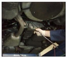
Now install the reinforcement brackets. The **driver's side** frame has two holes above the rear portion of the lower a-arm. Use the flange-headed bolts and place the head on the inside of the frame facing out. Take the black bracket marked '**D**' and place it up against frame as shown. The '**D**' sticker will end up against the frame, with the gusset towards the ground. Use the lock washers and lock nuts provided. Assemble with 14mm wrenches **and leave loose**, **DO NOT TIGHTEN**.
