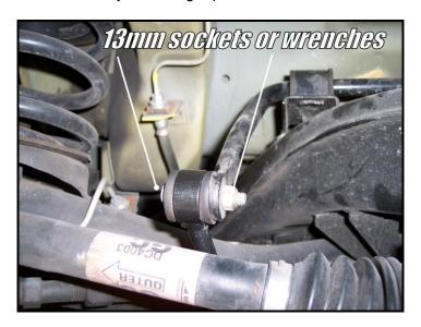
6) Undo the saddle brackets by removing 1 bolt per bracket using a 13mm socket. Simply rotate the bracket up and it will become detached from the cradle frame.
