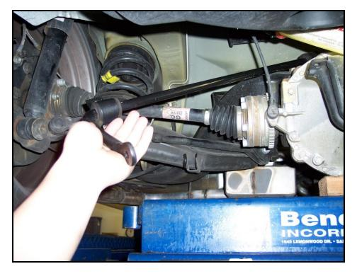
8) Set the Hotchkis sway bar next to the stock sway bar for proper orientation.
