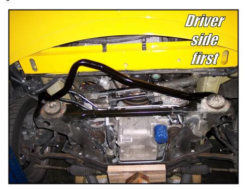
13) After the bar is in position, lube the inside hole of the Hotchkis polyurethane bushings with the included grease.
