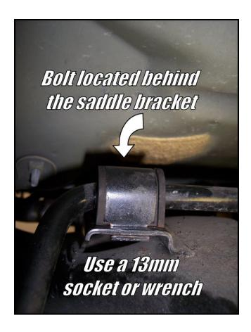
7) Remove the stock sway bar from the vehicle through either side of the differential.
