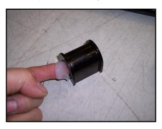
10) Open the bushing and push it over the bar. Make sure the flat side is facing down and the split is facing toward the front.
