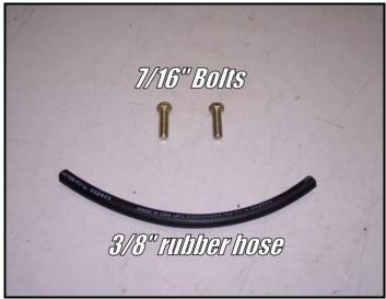
Now, clamp down on the other soft transmission line. Loosen the hose clamp using a 6mm socket. Then disconnect the soft hose from the hard line slowly. Once disconnected, connect the other end of the 3/8" hose to the hard line. Insert the 7/16" bolt into the soft transmission line and release the pinch-off pliers. The end result should look like the following picture.
