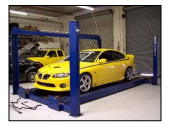
2) Support the Rear differential using a transmission jack or a center jack equipped on some 4-post lifts.
