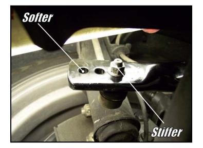
18) You are now finished with the Hotchkis front sway bar installation! Make sure that all hardware is fully tightened. On to the Hotchkis rear sway bar installation.
