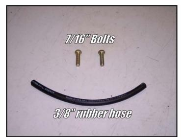
Now, clamp down on the other soft transmission line. Loosen the hose clamp using a 6mm socket. Then disconnect the soft hose from the hard line slowly. Once disconnected, connect the other end of the 3/8" hose to the hard line. Insert the 7/16" bolt into the soft transmission line and release the pinch-off pliers. The end result should look like the following picture.
