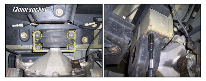
4) Slowly lower the transmission jack and let the differential and rear cradle frame tip downward.
