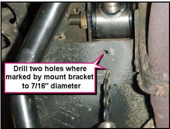
Drill out the holes for the brackets to 7/16" diameter. To accurately determine the location of the holes the end links must not be loose enough to move left or right. Make certain the axle is at its normal driving height for an accurate fit.
