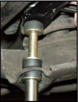
13) Re-check all hardware for tightness. Cover the zerk fittings in the brackets with the grease caps that came attached to the brackets. You are finished with the front sway bar installation
