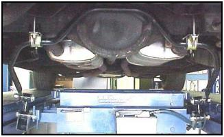
7) Snug down the hardware connecting the end links and brackets to the bar. **Do not** fully tighten the hardware at this stage. You should still be able to rotate the end links without difficulty.
