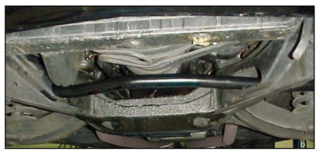
8) Use the grease pack provided to put a heavy coat of grease on the inside of the sway bar bushings. Place the bushings over the bar with the cut in the bushing towards the rear of the vehicle. Push the bushing retainer brackets into place on the bar and bolt them into place using the stock mounting hardware in the front holes only. **Do not** tighten the stock hardware.
