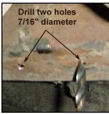
8) Once the holes are drilled, use a coat hanger to loop around one stud on the retainer bracket. Slide the bracket in through the rear end of the frame until the studs fall through the holes. Hold one stud and push the other stud back through the hole to slide the coat hanger loop off the stud.
