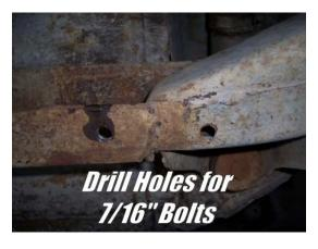
Once the holes are drilled, grab a 7/16" x 1.25" bolt (longer) and a 7/16" washer. Using a telescoping magnet wand, fish the bolt and washer through the box tubing and set the bolt into it's drilled out hole.
