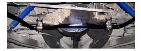
» Use the grease pack provided to apply a heavy coat of grease to the inside of the sway bar bushings. Place the bushings over the bar. Push the brackets onto the sway bar bushings.
