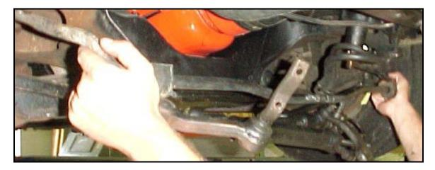
Leave the steering loose for installation of the Hotchkis sway bar at a later step.
