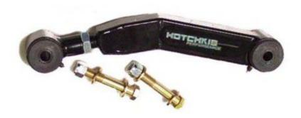
Adjustable upper trailing arm, to help eliminate pinion angle vibrations!
