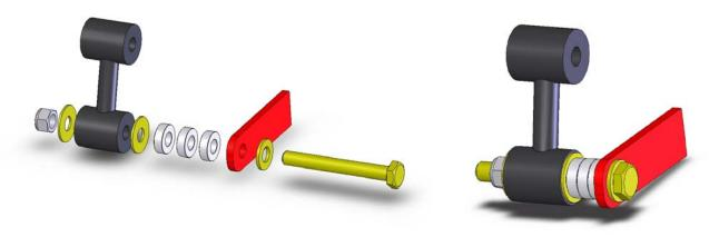
» Install the Clevis Bracket onto the dogbone endlink. Lightly tighten.
