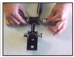
5) Hang the sway bar from the u-bolts on the axle. Slide the axle mount bracket over the ends of the u-bolts. Hold the sway bar up into place with the bushing retainer brackets mounted to the axle bracket.
