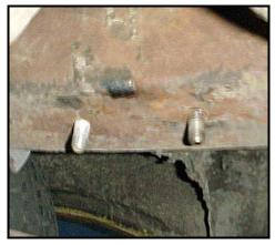
9) Rotate the sway bar so that you can bolt the brackets up to the stud plate in the frame using the 7/16" **hardware from kit #T1719**. You will only be using four of the nuts and the four smaller washers on the studs. *The four additional nuts and washers are extra hardware not used on this kit and may be discarded.* Tighten the nuts on the brackets and the end link hardware. Torque the end link hardware to 30ft/lbs.
