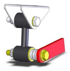
To accurately determine the location of the holes, the end links must NOT be loose enough to move left or right. Make certain the axle is at its normal driving height for an accurate fit. With the hardware lightly tightened, you can now rotate the bar up, so that the brackets are resting against the frame. Make sure both clevis brackets lay in the center of the frame. Position the clevis bracket onto the frame so that it will be possible to use either hole on the sway bar end.
