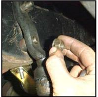
12) Check that all hardware is tight. Cover the grease fittings using the zerk caps provided. Remove the jack stands and move on to installing the rear sway bar!
