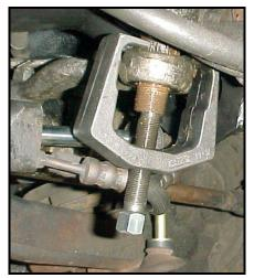
Note the position of the gearbox teeth and pitman arm to maintain proper steering when re-installing the pitman arm in a later step!
