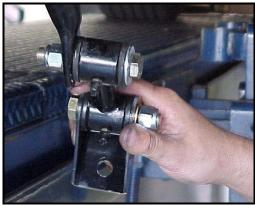
7) With the hardware loosely tightened you can now rotate the bar up, so that the brackets are resting against the frame. Once the brackets are in place use a scribe or similar tool to mark each hole for drilling. Drill out the holes for the brackets to 7/16" diameter. To accurately determine the location of the holes the end links must not be loose enough to move left or right.
