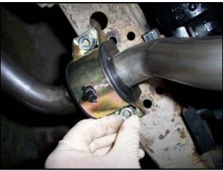
10) You can now fully tighten the endlink nuts & bolts. Tighten endlink until the bushing bulges to the same diameter as the washers.
