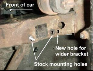
6) Install the included endlinks as shown below. Leave the endlinks loose for now, this will allow you to maneuver the bar more easily.
