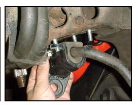
3) Remove the bolts holding the idler arm to the frame. Use a **1-5/16**" **socket or wrench** to remove the retaining nut attaching the pitman arm to the gearbox. Use the pitman arm puller to free the pitman arm from the gearbox.
