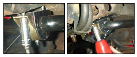
The driver's side bracket mounts inside of the power steering bracket included with the Hotchkis kit. Slide the retainer bracket into place over the bolts and tighten the bracket into place.
