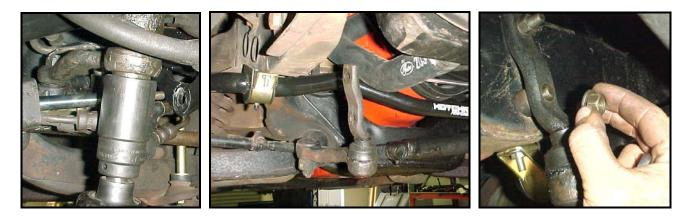
11) **Cars with power steering** should re-attach the power steering cylinder to the new bracket.
