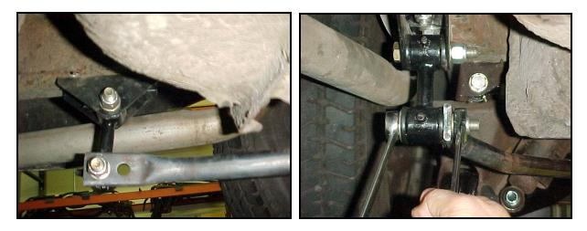
You can also adjust the stiffness of the bar by changing the hole the end link mounts to. The hole nearest to the end of the bar softens the bar stiffness by lengthening the bar. The hole furthest from the end of the bar stiffens the bar by shortening the length of the bar.
