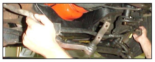
Leave the steering loose for installation of the Hotchkis sway bar at a later step.
