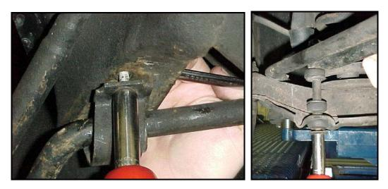
**Cars with power steering** will require that the power steering cylinder be unbolted from the bracket on the driver's side of the vehicle.
