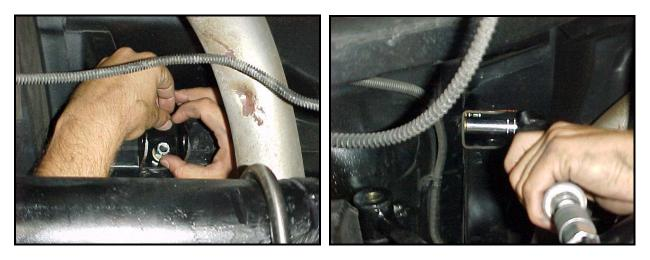
14) Re-attach the end links to the brackets, and tighten all attaching hardware on the end links. Torque the end link hardware to 35 ft/lbs
