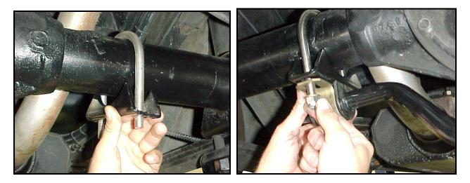
10) Use the Anti-Seize provided in hardware kit #T1722 to apply a small amount on the u-bolt threads. This will prevent damage to the nylock nuts when tightening or possible damage to the u-bolts. With the bar centered on the axle tighten the u-bolt hardware to 35-40 ft-lbs.
