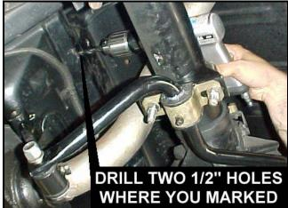
Drop the stud plate in from the passenger compartment through the holes. **Place one of the large washers provided over the lower stud on the plate**. This will act as a shim. It is also *suggested* to apply a ring of silicone gasket sealer to the edges of the holes and the stud plate to act as a water sealant.
