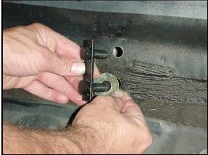
13) Remove the triangle brackets from the end links. Attach the brackets to the stud plate with the large end of the bracket closest to the ground. Tighten the hardware holding the bracket in place.
