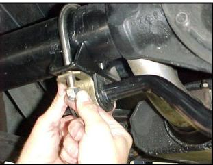
10) Use the Anti-Seize provided in hardware kit #T1722 to apply a small amount on the u-bolt threads. This will prevent damage to the nylock nuts when tightening or possible damage to the u-bolts. With the bar centered on the axle tighten the u-bolt hardware to 35-40 ft-lbs.
