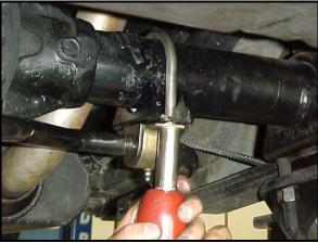
11) Rotate the sway bar into place with the triangle brackets up against the body. Use a scribe or other marking tool to mark the locations of the holes on the body matching the bracket. <u>Drill out</u> two 1/2" diameter holes on each side to match the bracket locations.
