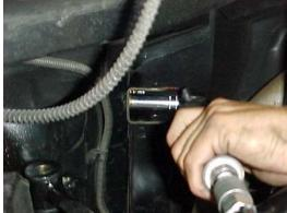
14) Re-attach the end links to the brackets, and tighten all attaching hardware on the end links.
