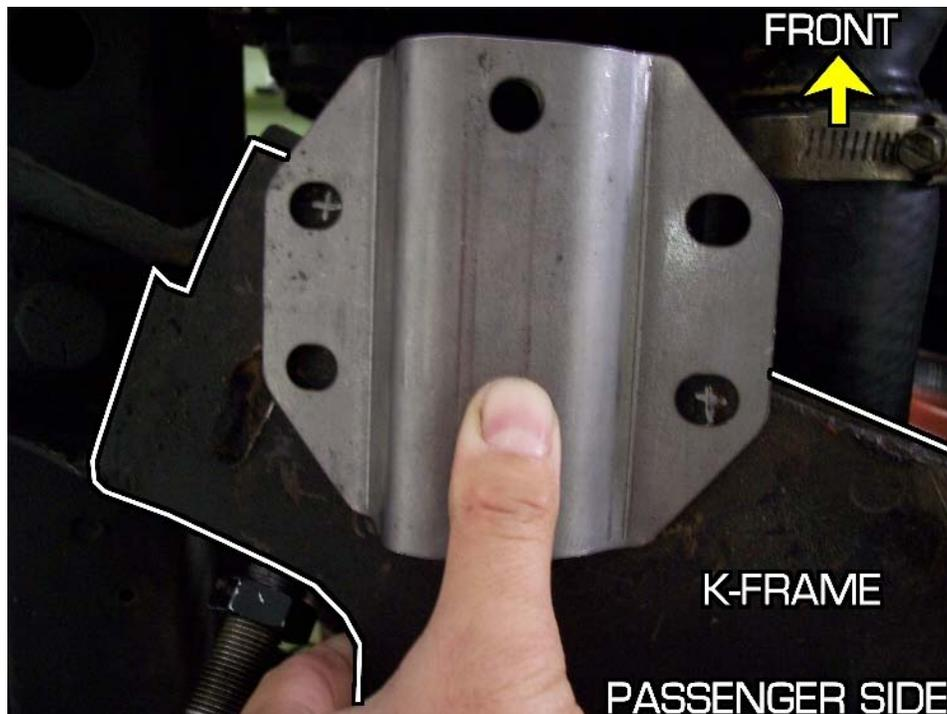
Use a paint marker to mark where the holes are as well as the outer edges that mate with the k-frame. (Picture shows bracket disconnected from the sway bar for clarity purposes.)
