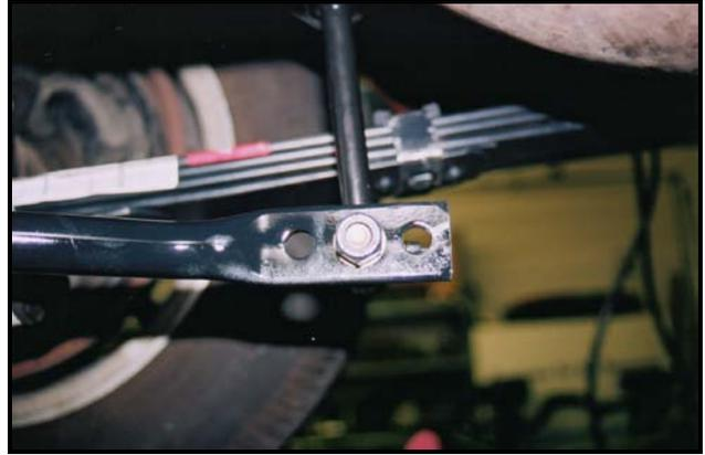
In the above picture the hole to the left is stiffer and the hole to the right is softer. Check that all attaching hardware is tight. Make certain the zerk fitting caps are covering the grease fittings. Lower the car from the jack stands and you're done!
