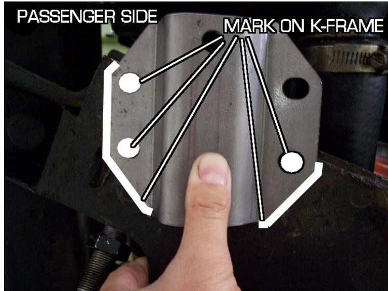
7. Once the k-frame is marked, use an angle grinder with a sand paper attachment to remove all of the paint and grime on the areas previously marked. What we are doing is cleaning the area that is going to be welded. You will also need to sand the bushing retainer bracket in the mating areas too.
