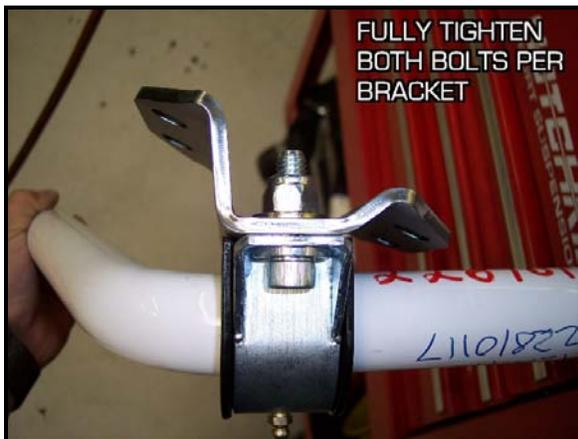
Now you can raise the bar up until the bushing retainer brackets mate flush to the k-frame bottom surface. Make sure the center section of the sway bar is not contacting any part of the k-frame. Bushing retainer bracket should be positioned similar to the picture below. The white outline depicts the k-frame. (Picture shows bracket disconnected from the sway bar for clarity purposes).
