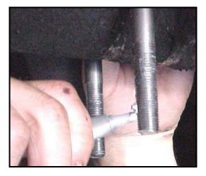
9) Make certain that the rear axle is at normal ride height to establish the proper orientation of the sway bar. Tighten the u-bolt hardware to mount the sway bar brackets to the axle. At this point you can now adjust the stiffness of the sway bar. Change the end link mount to the hole in the end of the bar to change the stiffness of the bar.
