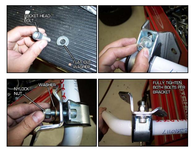
Now you can raise the bar up until the bushing retainer brackets mate flush to the k-frame bottom surface. Make sure the center section of the sway bar is not contacting any part of the k-frame. Bushing retainer bracket should be positioned similar to the picture below. The white outline depicts the k-frame. (Picture shows bracket disconnected from the sway bar for clarity purposes.
